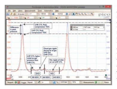
We always have to look for differences or anomalies between known good signals and here we can see good turbulence from both cylinders during the exhaust stroke indicating good airflow dynamics but a definite reduction in turbulence of the air flow during LHF cylinder intake stroke. We can also identify the early and prolonged opening of LHF cylinder inlet valve in comparison to the reference waveform and the reduction in peak vacuum, all linked to the condition revealed below.
