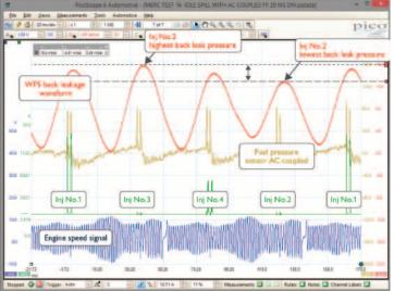
Traditionally the volume of "back leakage" has been measured using graduated collection bottles, while monitoring both the rate and amount of "fill" during cranking or pre-set running conditions. This test will always remain relevant as manufacturers often specify the volume of back leakage against time, but the WPS500X will reveal intermittent issues under all driving and test conditions.
