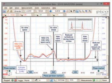
150 rpm above idle but near 50% misfire during relative compression test at 200 rpm). Looking back at the testing carried out the inlet valve could only have been marginally mis-seated as no misfire could be detected using cylinder cut or emission methods, yet the PCM had identified an anomaly with crankshaft rotational speed as did the relative compression test. The engine has since been reassembled with an inlet valve clearance of 0.12 mm and all is well with no misfire count or code apparent.
