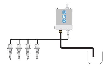
Run the back leakage test with WPS500X and see so much information clearly revealed.
